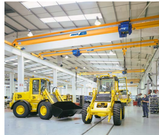
Type E monorail hoists on type ELV single girder overhead travelling cranes.
