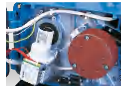
Geared limit switch with up to 8 contacts for cut-off at predefined positions
